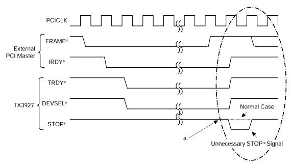
Figure 1 Unnecessary assertion of the STOP\* signal
